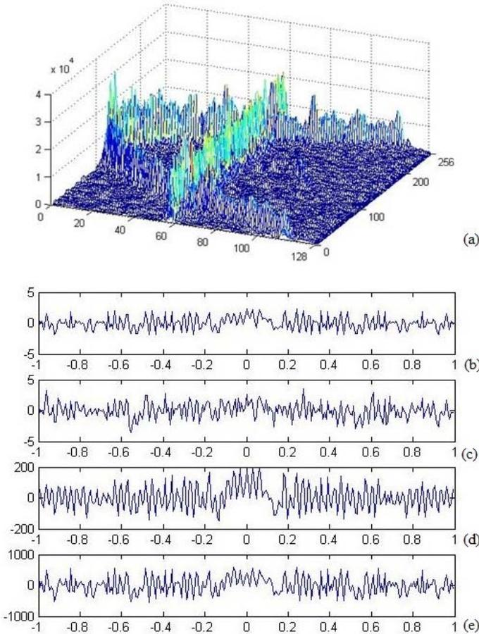
**Fig. 1** (a) CTFWD of the multicomponent noisy signal (3), (b) Original multicomponent signal (3), (c) Noisy signal (3), (d) The estimated signal obtained by using the state-of-the-art IF estimation algorithms from [2, 5], (e) The estimated signal obtained by using the modified IF estimation algorithm.
