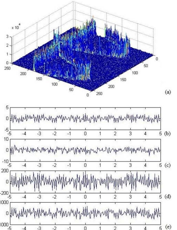
**Fig. 2** (a) CTFWD of the multicomponent noisy signal (4), (b) Original multicomponent signal (4), (c) Noisy signal (4), (d) The estimated signal obtained by using the state-of-the-art IF estimation algorithms from [2, 5], (e) The estimated signal obtained by using the modified IF estimation algorithm.
