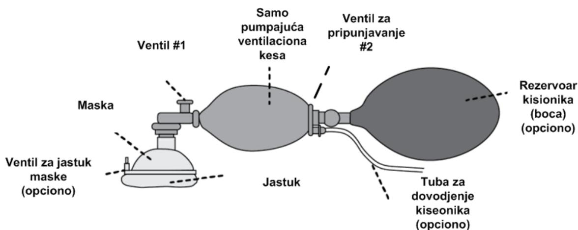
Figure 2: The principle of operating AMBU handheld breathing apparatus
